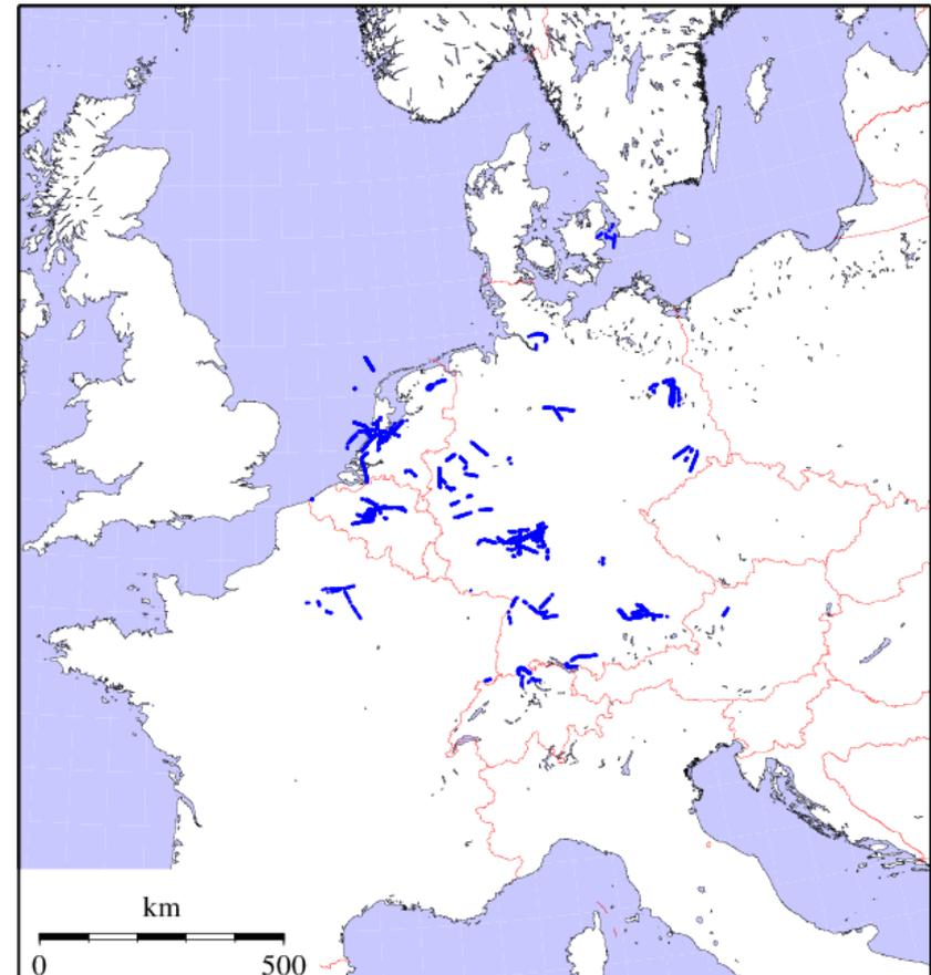
Example of 15 minutes of derived Wind and Temperature observations from Mode-S EHS data of a day in August 2012 over Western Europe, source MUAC, processed by KNMI
