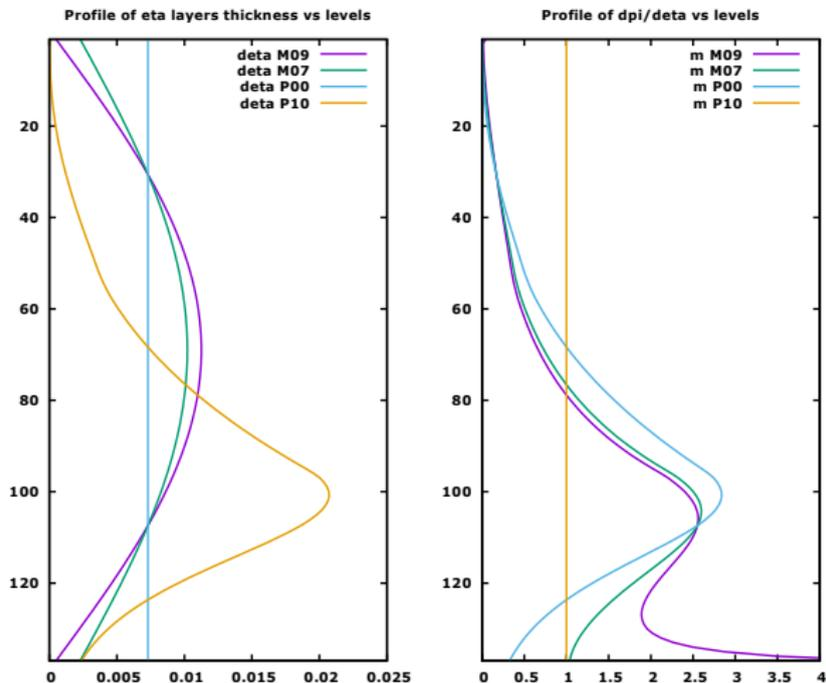
Profiles of layer thickness  $\delta\eta$  and  $\frac{\partial\pi}{\partial\eta}$  vs levels index for various definitions of  $\eta$  coordinate
