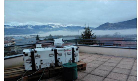
Scanning Doppler wind lidar in Passy experiment
