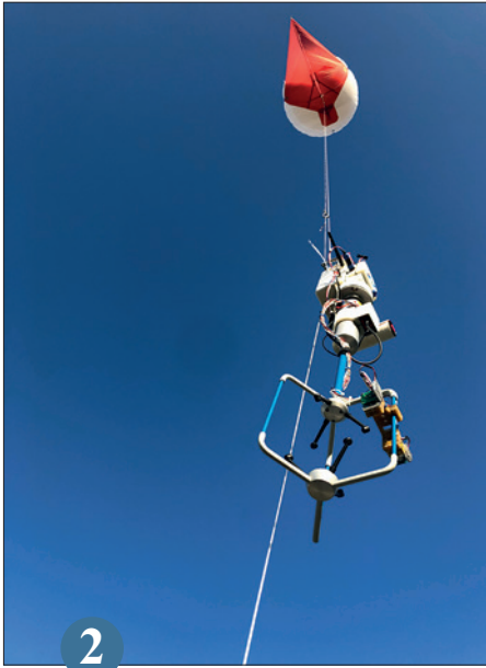
Turbulence probe under tethered balloon during a test flight. The mini spectrometer that measures fast humidity is installed on the right arm of the sonic anemometer.
