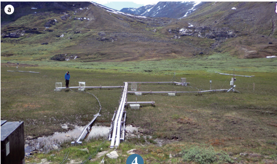
(a) View of the fen ( 64^{\circ}7'51.5''N , 51^{\circ}23'10.5''W ) in July 2017 with the greenhouse gas fluxes measuring tools: eddy flux tower and automatic chambers
