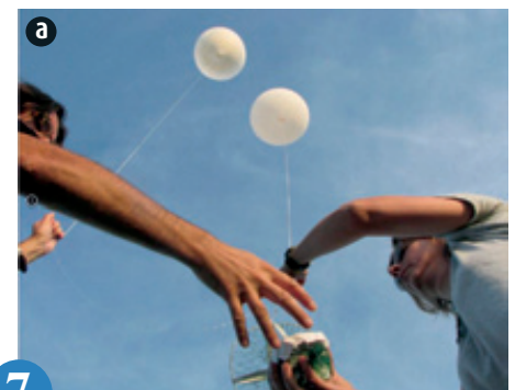
a: Release of a recoverable radiosonde with dual balloons during the BLLAST 2011 campaign. b: Sample simulations of dual-balloons recoverable radiosondes during the PASSY 2015 campaign
