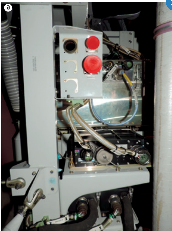
▲ a: The Real Time Transmission Unit (RTTU) is a gateway between the IAGOS system and the on-board Satcom telecommunication system. b: The IAGOS system and the Real Time Transmission Unit (RTTU) are located in the technical hold. The Lufthansa Technik electrician carefully follows the specifications for modifying the electrical wires connecting the RTTU to the Satcom (Satellite communication).
