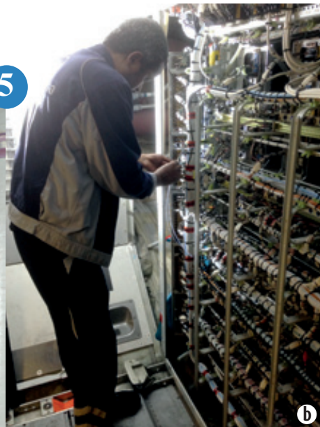
▲ a: The Real Time Transmission Unit (RTTU) is a gateway between the IAGOS system and the on-board Satcom telecommunication system. b: The IAGOS system and the Real Time Transmission Unit (RTTU) are located in the technical hold. The Lufthansa Technik electrician carefully follows the specifications for modifying the electrical wires connecting the RTTU to the Satcom (Satellite communication).
