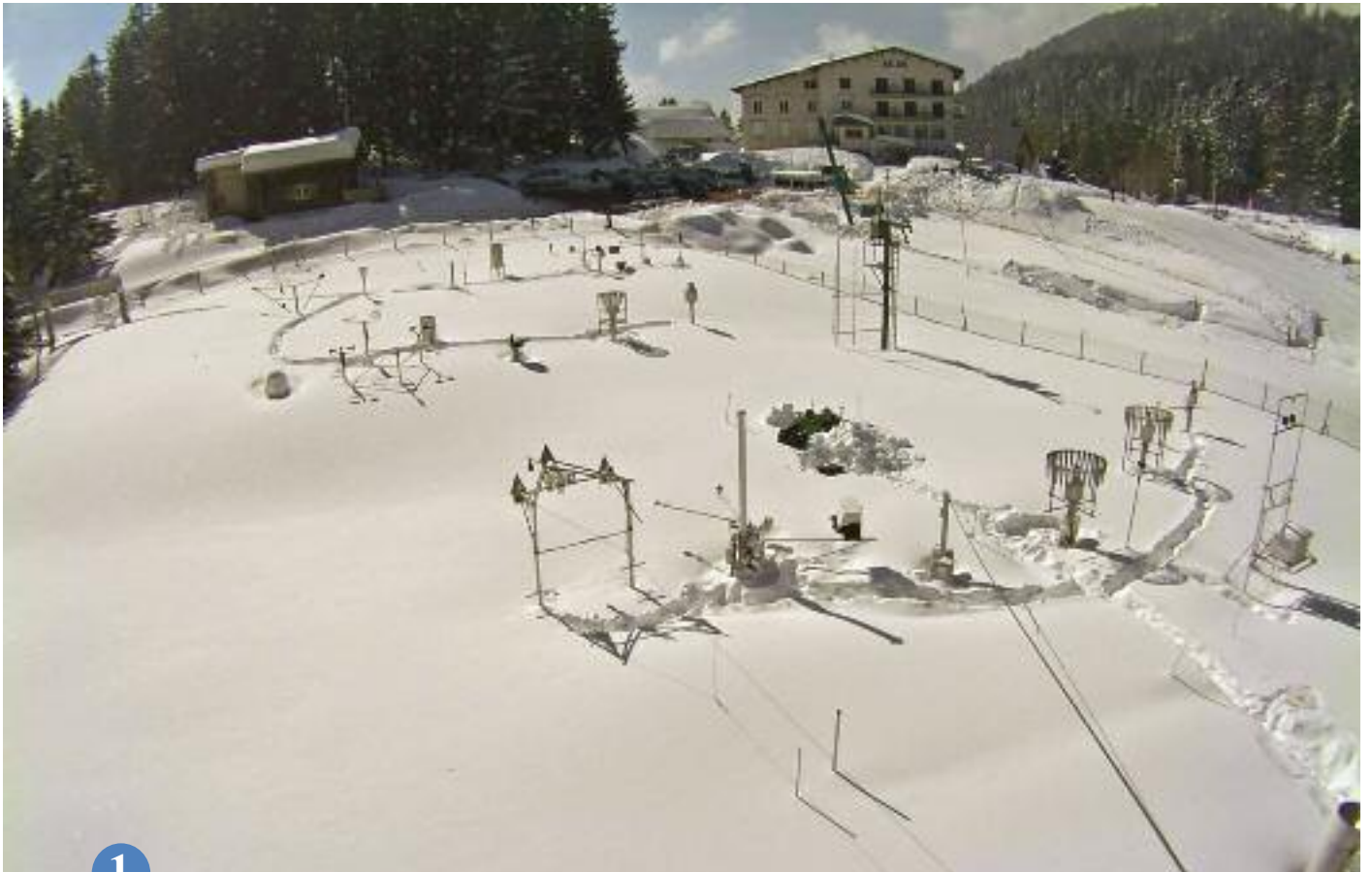
Overview of the instrumental plot of the experimental site at Col de Porte, including sensors deployed for the WMO-SPICE project.
