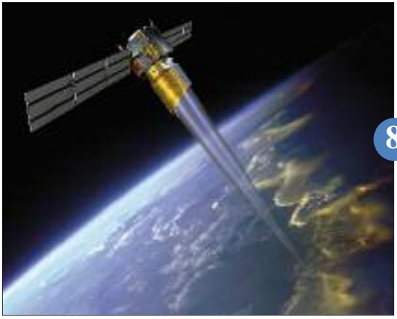
▲ Artist view of the AEOLUS satellite pointing its laser beam down towards the atmosphere.
