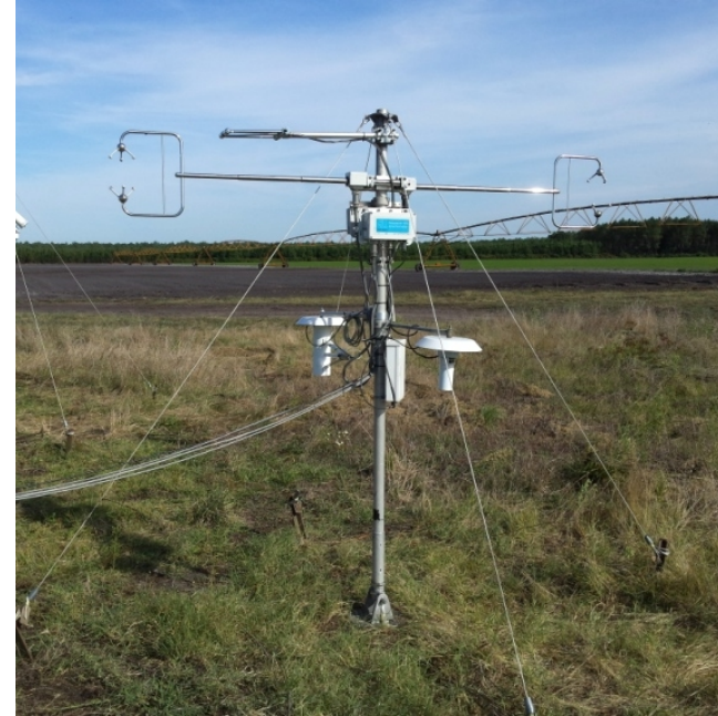
Gill HS50 sonic anemometers at 2m agl
