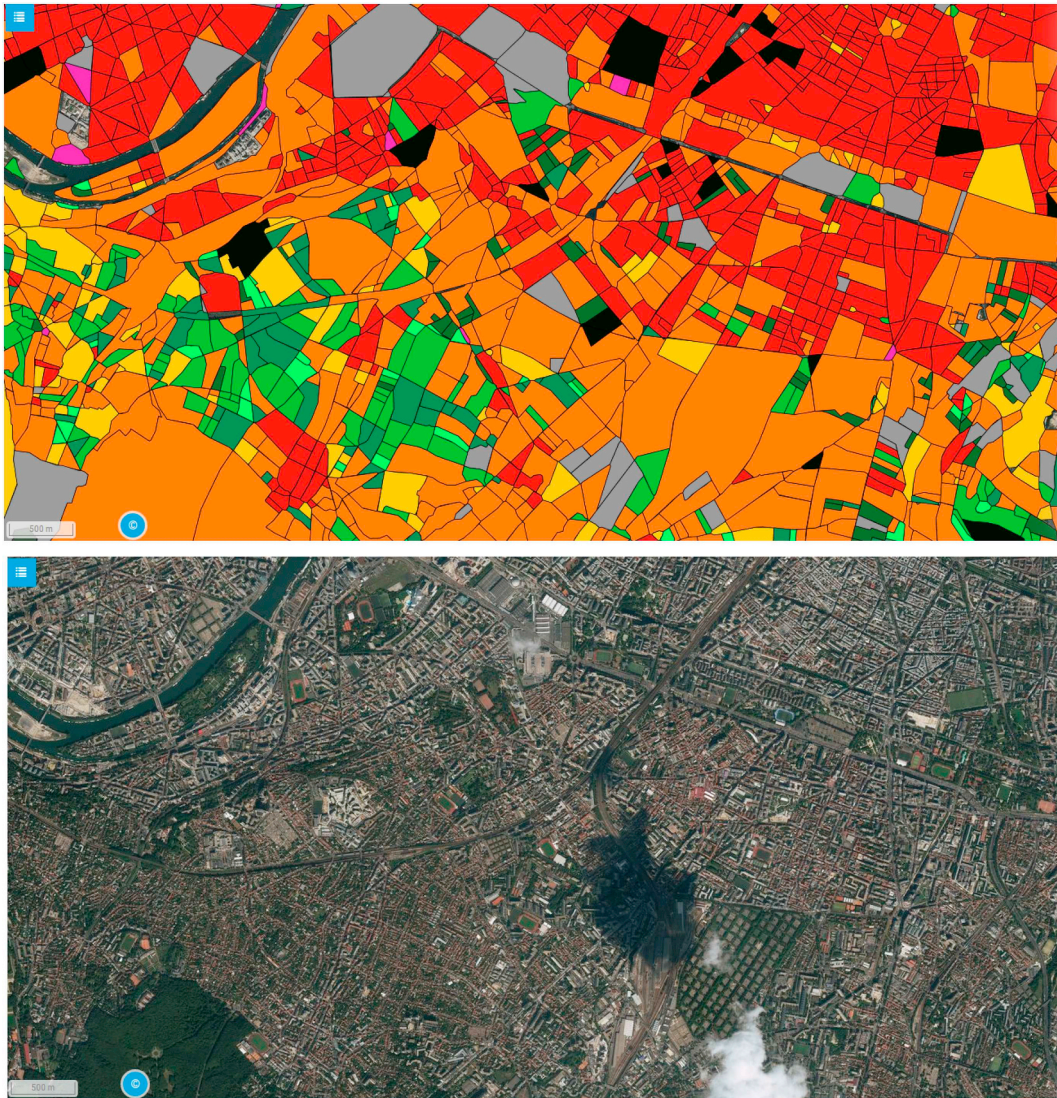
Fig. 2. Dominant building type and aerial map (ESRI World Imagery) at the RSU scale for a district of Paris. Code of colours corresponds to Table 3 (Other type is represented with a transparent colour).
