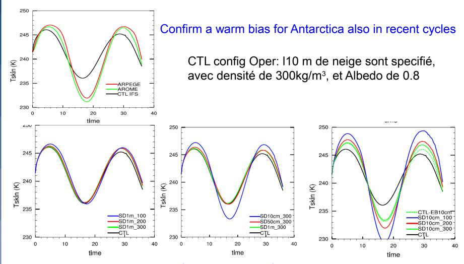
The snow thermal properties and the surface roughness specified in the model are crucial to enhance the amplitude of the diurnal cycle
