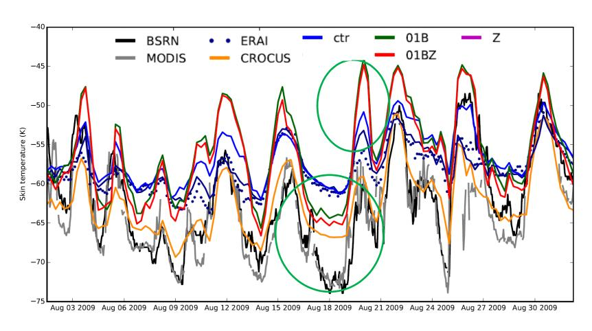
Consistent with SCM and offline, amplification of the Tskin variations, due to less thermal inertia, but also less sensitivity to roughness in coupled mode
