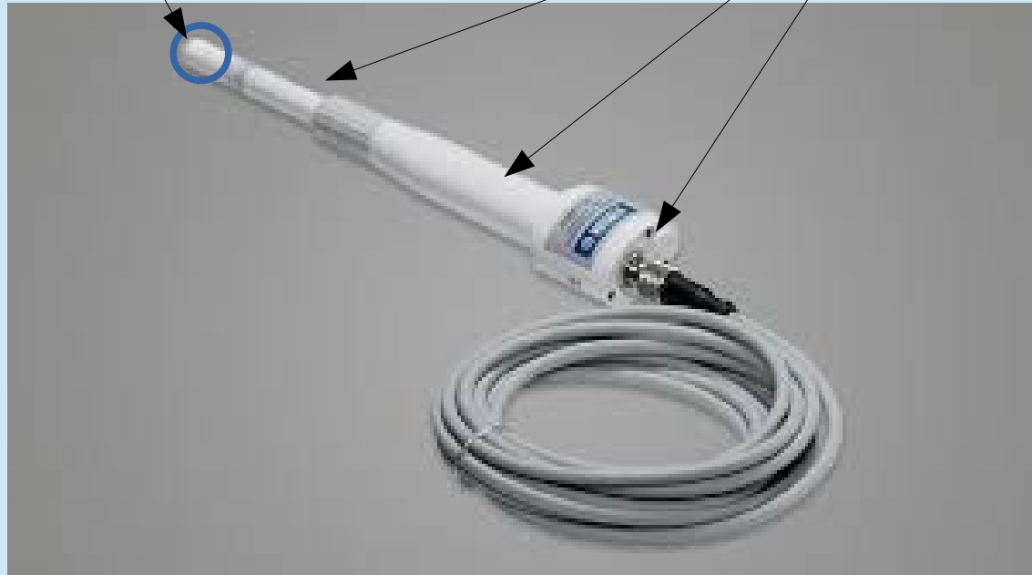
A typical commercial hygrometer (Vaisala HMP155)
