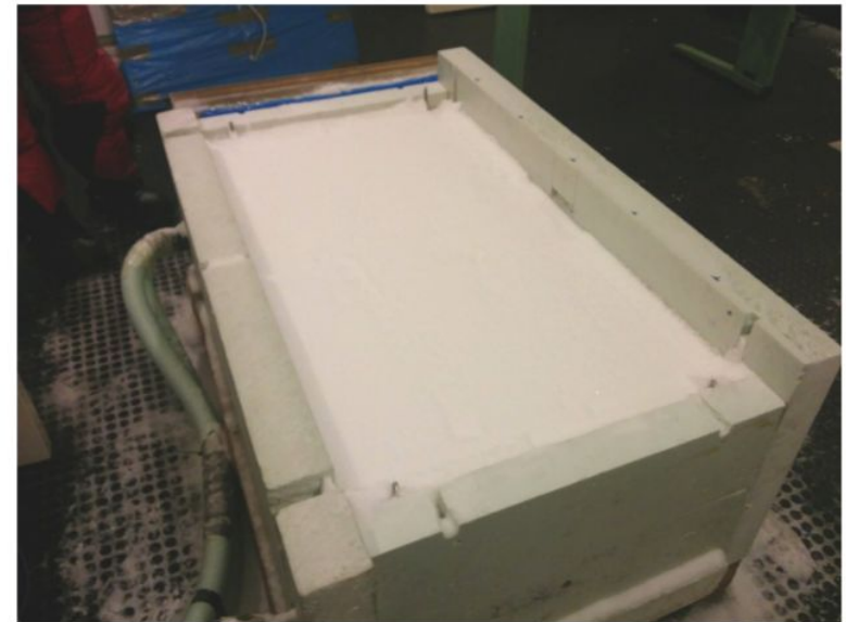
(a) With polystyrene side walls removed to show snow sample and copper plates. (b) Seen from above with upper plate removed to perform SMP measurement.
