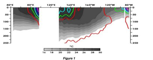
Equatorial mean structure within the first 250 meters over the tropical Indian-Pacific sector (1993-2001) for a) MERCATOR POG05B simulation and for b) the observations (World Ocean Atlas 2001). Grey shading represents the mean temperature section between 16°C and 30°C. 34, 34.25, 34.5, 34.75, 35 iso-salinity are represented with red, green, light blue, blue and purple solid lines respectively.
