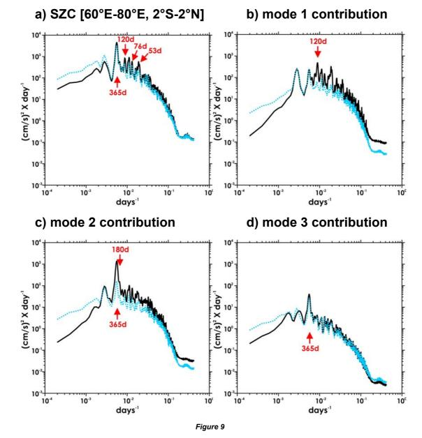
Mean conservative spectrum [60°E-80°E, 2°S-2°N] of the ILIN Surface Zonal Current (SZC) estimated by autocorrelation for a) the total ZSC, b-d) the contribution of the 3 gravest baroclinic modes respectively. The plain black (dashed blue) line respectively corresponds to the control experiment ('no reflection' experiment).
